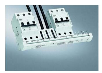
Connection of the supply leads coming from above with crosssections of up to 35 mm<sup>2</sup> to 5ST2 144 busbar over additional terminal 5ST2 157.
