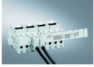
Simultaneous connection of the supply leads coming from below with cross-sections of up to 35 mm² and 2-pole 5ST2 143 busbar over 5ST2 166 terminal.
