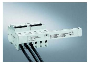
Simultaneous connection of the supply leads coming from below with cross-sections of up to 25 mm² and the three-pole 5ST2 144 busbar to the combination terminal of the miniature circuit-breaker.
