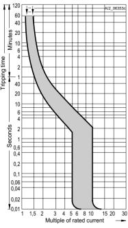
• General line protection, especially advantageous with higher starting currents (lamps, motors, etc.,).
