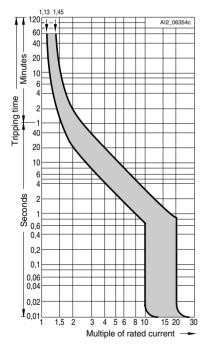
The tripping range has been matched to applications involving equipment generating significant pulses (transformers, solenoid valves) In the case of different ambient temperatures, the current values of the delayed tripping operation change by approx. 5% per 10 K temperature difference > for temperatures lower and < for temperatures higher than 30 °C.
