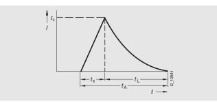
Current path when switching fuse links
