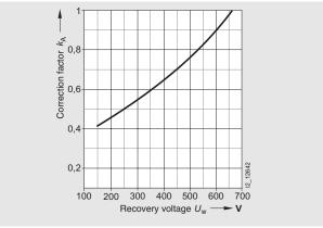
Correction factor  $k_A$  for breaking  $I^2t$  value
