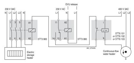
In mixed operation of electric hot water and electric storage heaters, the priority switch interrupts the charging procedure of the storage heater if hot water is required during the low-tariff time, thus limiting the connected load.
